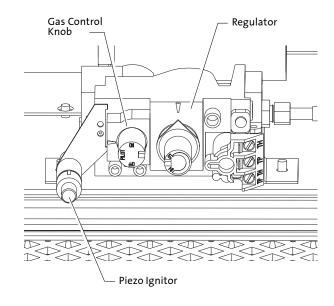
Figure 30. GI425 Controls - Gas Valve and Regulator.
